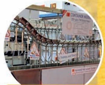
Hot Water Scalding
