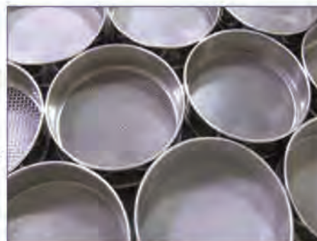
Figure 3. Sieves of varying sizes used to separate a mash feed sample by particle size. Image courtesy Gilson Company, Inc.
